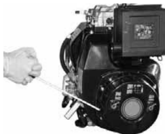
3: Let the starter cord recoil back into position, then pull starter cord hard.
