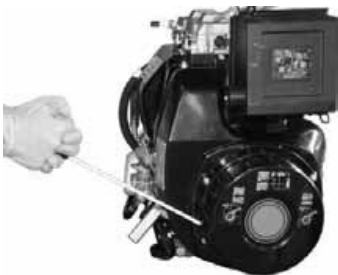
1: Pull the rope starter until the engine comes up to compression.
