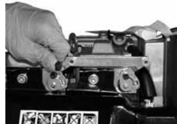
2: Pull decompression levers over. The starting position is correct only if the levers remain engaged.
